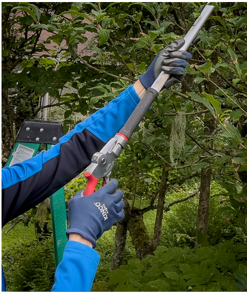
Extension by-pass pruners have a big handle for operation and enable reaching a bit higher without a ladder.
