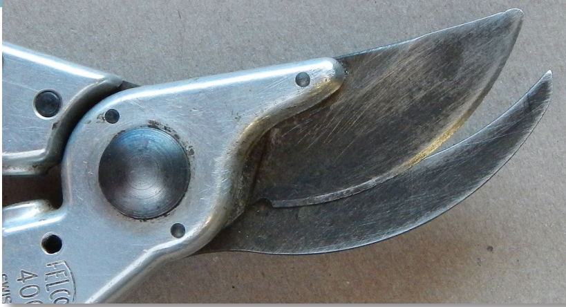
Left: By-pass type cutting tool. Above: Anvil type cutter. Instead of slicing a clean cut through plant parts, it smashes them causing damage. You can see the gap that wears over time making the tool ineffective.
