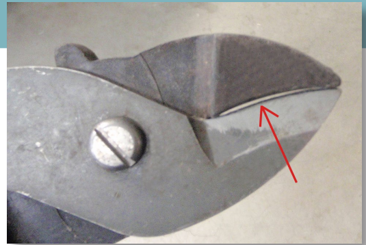
Left: By-pass type cutting tool. Above: Anvil type cutter. Instead of slicing a clean cut through plant parts, it smashes them causing damage. You can see the gap that wears over time making the tool ineffective.
